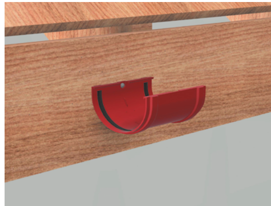
Figure 28 – Mounting PREMIUM and STANDARD connectors on the fascia
