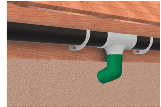
Figure 40 – Installing the elbow on the outlet's drain hole
