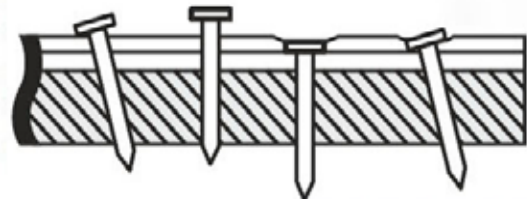
Fig. 3. An example of improper nailing for the installation of the product.
